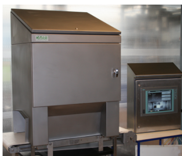
Fig. 1. The 6 wavelength inspection system. Camera box to the left and box for computer, network switch and power supplies to the left.
